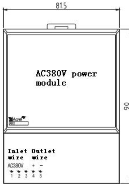
Figure 9 Outline dimensions of AC380 power module
